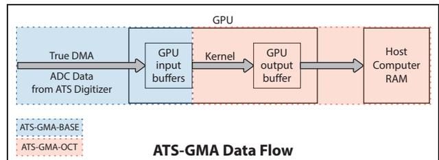
ATS-GMA-BASE is supplied with an example user application in source code. The application includes GPU kernels that use ATS-GMA-BASE to receive data, do very simple signal processing (data inversion), and copy the processed (inverted) data back to a user buffer. All this is done at the highest possible data transfer rate.
