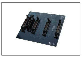
SyncBoard 860 is a board-level product that features clock buffering, clock distribution, trigger resynchronization and controlled impedance, equal length traces to deliver Positive Emitter Coupled Logic (PECL) level clock, trigger and initialization signals to each ATS860 in the system.
