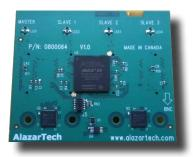
SyncBoard-9416 is a mezzanine board that connects to the Master/Slave connector along the top edge of the ATS9416 and sits parallel to the motherboard. For additional robustness, users can secure the SyncBoard-9416 to a bracket mounted on each of the ATS9416 boards.
