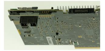
To further assist the user, AlazarTech will also include a very high quality 1 meter long PCI Express bus extension cable that will allow the ATS9626 to be brought out of the chassis and on to the bench, so various LEDs are visible.
