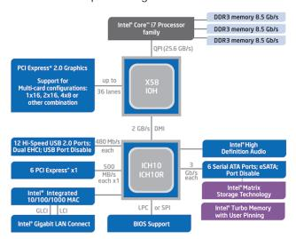
One of the advantages of this architecture is that the X58 chipset communicates directly with PCI Express slots, thereby reducing system latencies and increasing sustained throughput.
