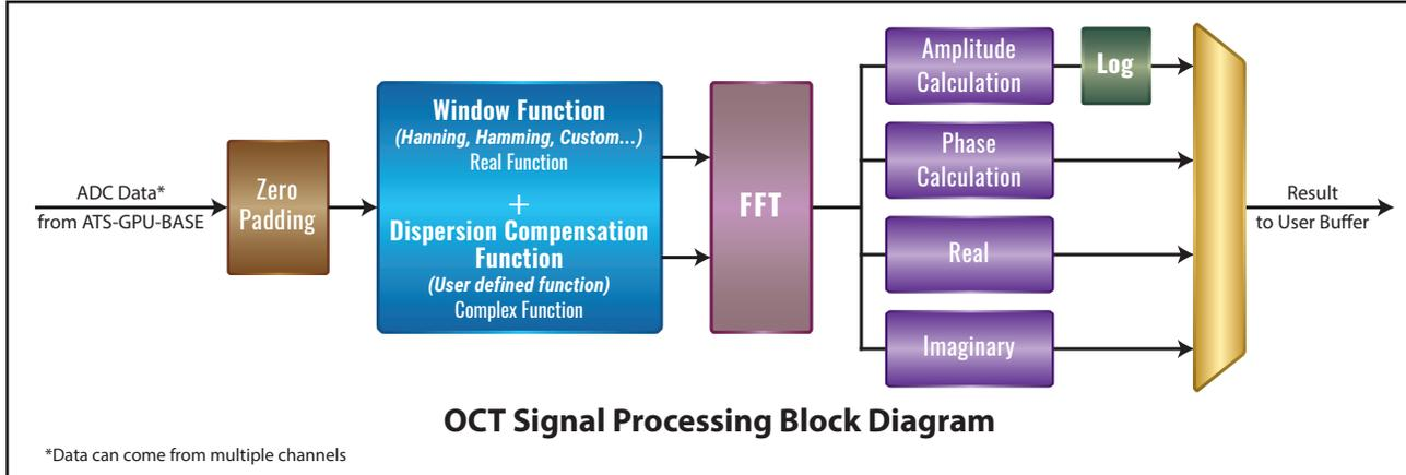
ATS-GPU-OCT is supplied with example programs in C/C++, Python, LabVIEW, and MATLAB that allows users to set-up the waveform digitizer parameters, set-up FFT parameters in the GPU, do the acquisition, and receive the FFT result buffer.
