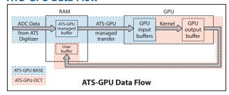
ATS-GPU-BASE is supplied with an example user application in source code. The application includes GPU kernels that use ATS-GPU-BASE to receive data, do very simple signal processing (data inversion), and copy the processed (inverted) data back to a user buffer. All this is done at the highest possible data transfer rate.
