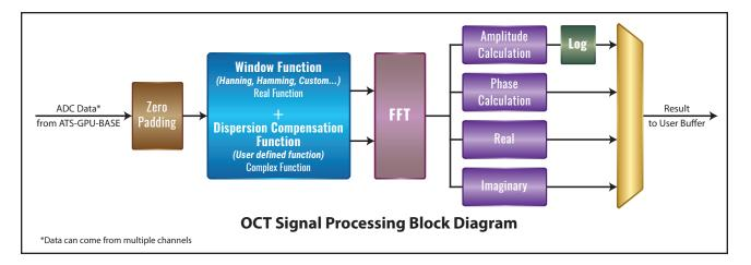
ATS-GPU-OCT is supplied with example programs in C/C++, Python, LabVIEW, and MATLAB that allows users to set-up the waveform digitizer parameters, set-up FFT parameters in the GPU, do the acquisition, and receive the FFT result buffer.
