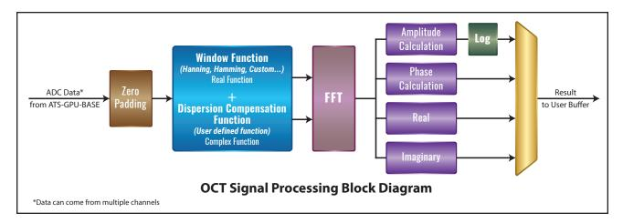
ATS-GPU-OCT is supplied with example programs in C/C++, Python, LabVIEW, and MATLAB that allows users to set-up the waveform digitizer parameters, set-up FFT parameters in the GPU, do the acquisition, and receive the FFT result buffer.
