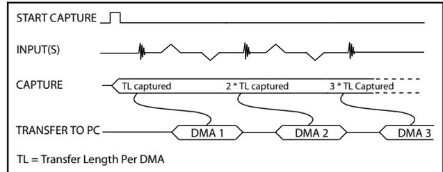
A BUFFER\_OVERFLOW flag is asserted only if the entire on-board memory is used up.
