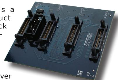
A Master/Slave system is guaranteed to sample simultaneously across all channels in that system. Triggering is also guaranteed to be simultaneous across all digitizers in the system, i.e. all boards will trigger on the same clock edge.
