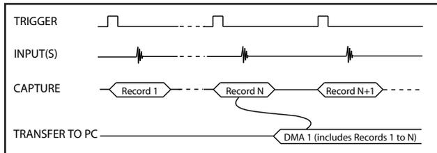
Note that a DMA is not started until RecordsPerBuffer number of records (triggers) have been acquired.
