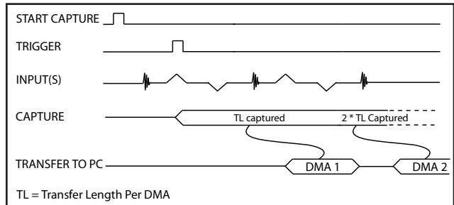
Triggered Streaming AutoDMA buffers do not include headers, so it is not possible to get trigger time-stamps.
