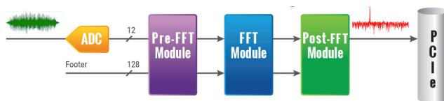
Up to 4096 point FFT length is supported. A user programmable complex windowing function can be applied to the acquired data before FFT calculation.
