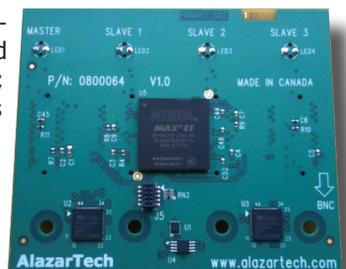
The Master board's clock, trigger and initialization signals are copied by the SyncBoard-9416 and supplied to all the Slave boards. This guarantees complete synchronization between the Master board and all Slave boards.
