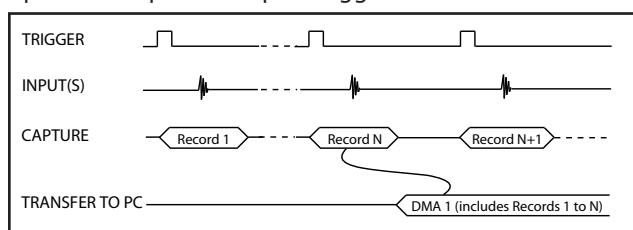
Note that a DMA is not started until RecordsPerBuffer number of records (triggers) have been acquired and written to the on-board memory.
