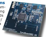
SyncBoard 9462 is a mezzanine board and plugs into the connector located along the top edge of the ATS9462 boards.
