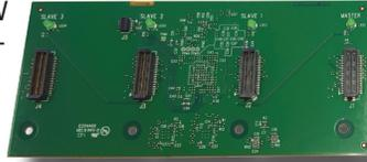
The 2x and 2x-W models allow a 2-board Master/Slave system; the 3x-W model allows a 2 or 3-slot Master/Slave system; and the 4x and 4x-W models allow 2, 3 or 4 board Master/Slave systems.
