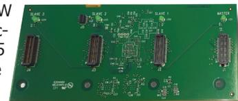
the on-board x8 or x16 slots by two slots. The -W SyncBoards are also a better solution from thermal point of view, as there is better air flow with 2-slot spacing.
