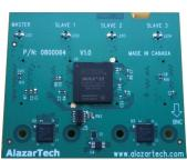
SyncBoard-9626 is available as a 2x or a 4x model: the 2x model allows a 2-board Master/ Slave system whereas the 4x model allows 2, 3 or 4 board Master/Slave systems.
