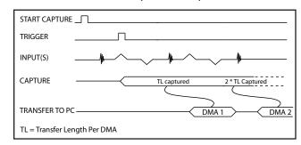
As in Continuous mode, the amount of data to be captured is controlled by counting the number of buffers acquired.
