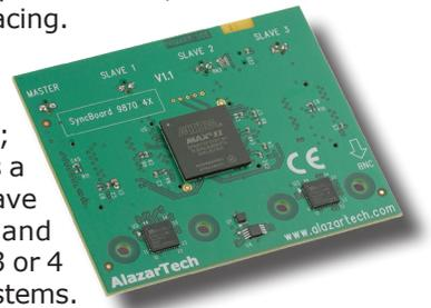
The Master board's clock and trigger signals are copied by the SyncBoard-9870 and supplied to all the Slave boards. This guarantees complete synchronization between the Master board and all Slave boards.
