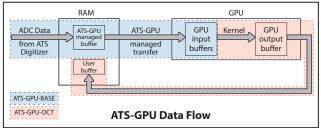
ATS-GPU-BASE is supplied with an example user application in source code. The application includes GPU kernels that use ATS-GPU-BASE to receive data, do very simple signal processing (data inversion), and copy the processed (inverted) data back to a user buffer. All this is done at the highest possible data transfer rate.
