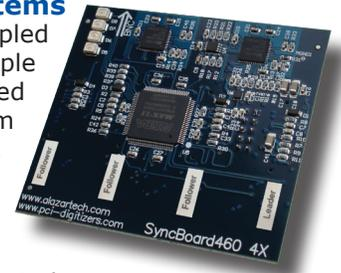
SyncBoard 9462 is a mezzanine board and plugs into the connector located along the top edge of the ATS9462 boards.
