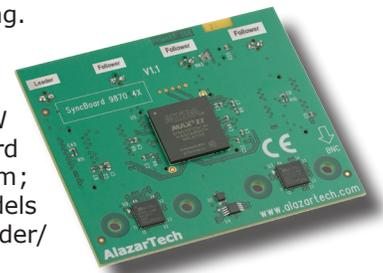
The Leader board's clock and trigger signals are copied by the SyncBoard-9870 and supplied to all the Follower boards. This guarantees complete synchronization between the Leader board and all Follower boards.
