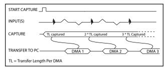
In this mode, data starts streaming across the PCI bus as soon as the ATS660 is armed for acquisition. It is important to note that triggering is disabled in this mode.
