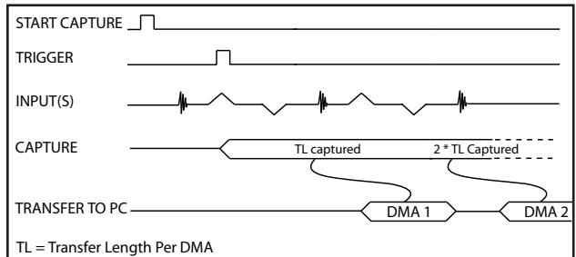
A BUFFER\_OVERFLOW flag is asserted only if the entire on-board memory is used up.
