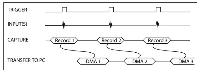
While Traditional AutoDMA can acquire data to PC host memory at the maximum sustained transfer rate of the motherboard, a BUFFER\_OVERFLOW can occur if more than 512 triggers occur in very rapid succession, even if all the on-board memory has not been used up.
