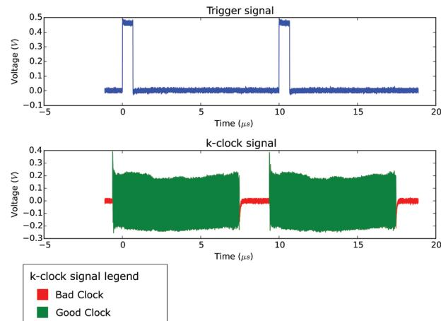
Users must set the trigger source to be External Trigger input (TRIG IN) when using OCT Ignore Bad Clock. The External Trigger must be set in TTL input range. If these two conditions are not met, the OCT Ignore Bad Clock circuitry will not function.
