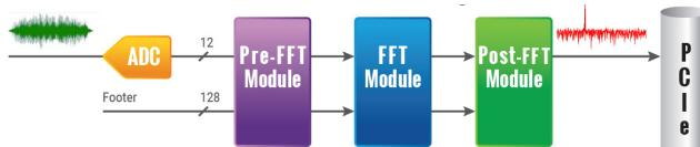
Up to 4096-point FFT length is supported. A user programmable complex windowing function can be applied to the acquired data before FFT calculation.
