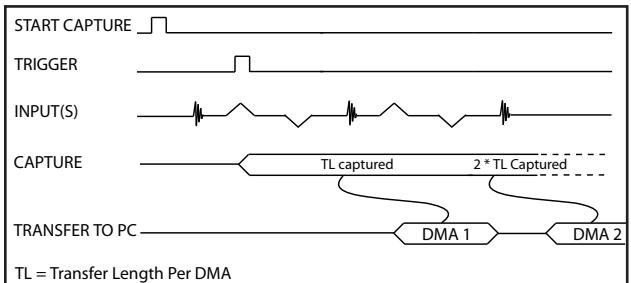
Triggered Streaming AutoDMA can easily acquire data to PC host memory at the maximum sustained transfer rate of the motherboard without causing an overflow. This is the recommended mode for RF signal recording that has to be started at a specific time, e.g. based on a GPS pulse.
