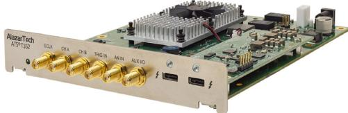
ATST352-OEM features two power connectors: a DC-jack that is used with an external AC-DC power supply; and a 2 pin locking Molex MiniFit 39-29-9029 connector that can be used in applications that require a more robust connection in OEM applications.
