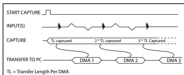
Continuous AutoDMA buffers do not include headers, so it is not possible to get trigger time-stamps. A BUFFER\_OVERFLOW flag is asserted only if the entire on-board memory is used up.
