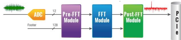
Up to 4096-point FFT length is supported. A user programmable complex windowing function can be applied to the acquired data before FFT calculation.
