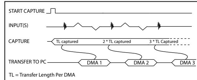
The amount of data to be captured is controlled by counting the number of buffers acquired. Acquisition is stopped by an AbortCapture command.
