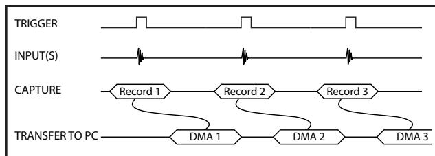
Data is returned to the user in buffers, where each buffer can contain from 1 to 8192 records (triggers). This number is called RecordsPerBuffer.
