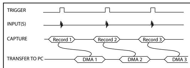
While Traditional AutoDMA can acquire data to PC host memory at the maximum sustained transfer rate of the motherboard, a **BUFFER\_OVERFLOW** can occur if more than 512 triggers occur in very rapid succession, even if all the on-board memory has not been used up.
