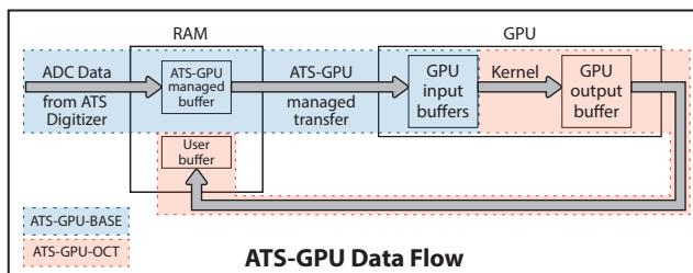
ATS-GPU-BASE is supplied with an example user application in source code. The application includes GPU kernels that use ATS-GPU-BASE to receive data, do very simple signal processing (data inversion), and copy the processed (inverted) data back to a user buffer. All this is done at the highest possible data transfer rate.
