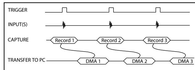
Data is returned to the user in buffers, where each buffer can contain from 1 to 8191 records (triggers). This number is called RecordsPerBuffer.
