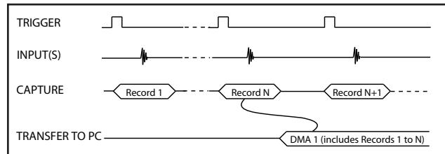
NPT AutoDMA buffers do not include headers. However, users can specify that each record should come with its own footer that contains a 40-bit trigger timestamp. The footer is called NPT Footer.
