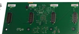
The Leader board's clock and trigger signals are copied by the SyncBoard-9440 and supplied to all the Follower boards. This guarantees complete synchronization between the Leader board and all Follower boards.
