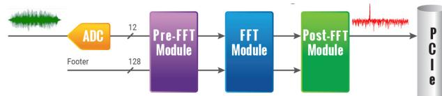
The complex FFT output is converted to magnitude in single precision floating-point format. A logarithmic output is also available.
