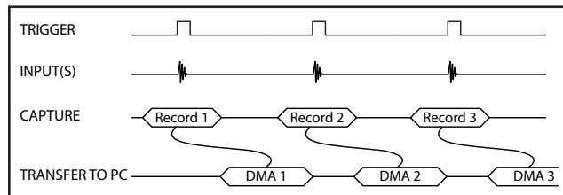
While Traditional AutoDMA can acquire data to PC host memory at the maximum sustained transfer rate of the motherboard, a BUFFER\_OVERFLOW can occur if the amount of memory that has been written into but not read out to PCIe bus exceeds the on-board memory size.
