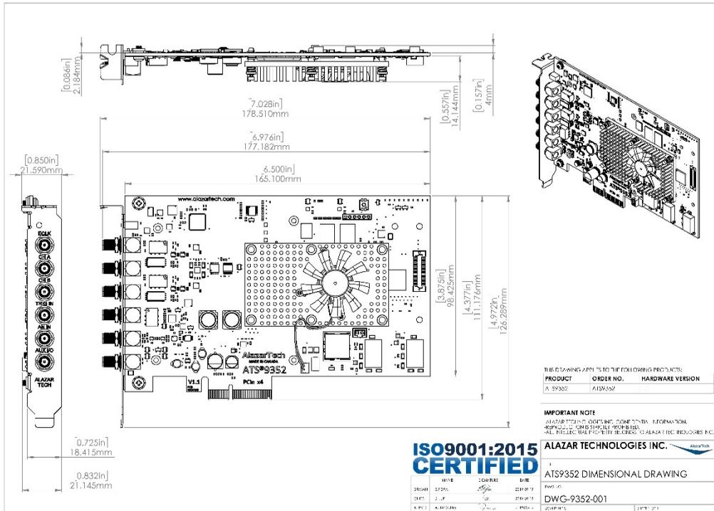
Figure 2 - ATS9352 Mechanical Drawing
