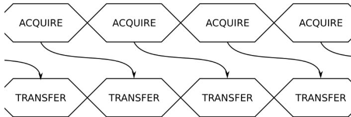
**Figure 6 - AutoDMA acquisition and transfer cycle**
