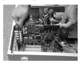
Always screw the digitizer bracket to the chassis in order to create a stable and robust connection to chassis ground.
