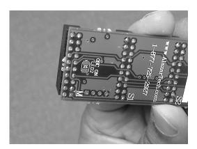
If you are installing fewer than the maximum number of digitizers supported by your SyncBoard, the unused SyncBoard connectors must be on the right-hand side of the digitizers, if you are facing the BNC connectors of the ATS310 digitizers.
