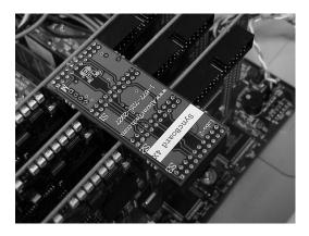
The presence of a SyncBoard is detected by the ATS310 driver when the ATSApi DLL is loaded. This DLL gets loaded when you run any application program written for ATS310. Examples of such application programs are AlazarDSO, one of the sample programs supplied with ATS-SDK or ATS-VI or any custom software written using ATS-SDK or ATS-VI.
