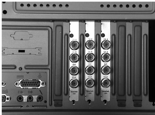
The connector on the SyncBoard that is labeled as “M” (Master), must be inserted into the Master/Slave connector of the left-most digitizer, if you are facing the BNC connectors of the ATS310 digitizers.
