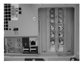
The connector on the SyncBoard that is labeled as "M" (Master), must be inserted into the Master/Slave connector of the left-most digitizer, if you are facing the BNC connectors of the ATS660 digitizers.
