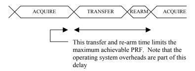
ATS660 solves this problem by providing dual-port memory. When operated in Multiple Record mode (Record Count > 1), a new record is being captured even while you read the previous one from the on-board memory.
