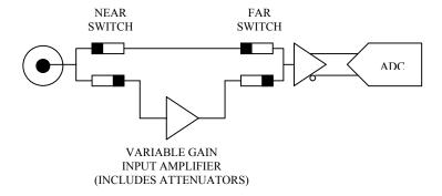
There are two DIP switches per channel: the one closest to the input BNC connectors is called the "Near Switch" and the one closest to the ADC IC is called the "Far Switch".
