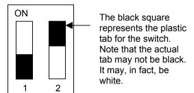
To set Amplifier Bypass Option for a channel, change the DIP Switch setting of the Near and Far switches for that particular channel to be as shown below:
