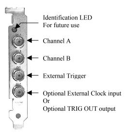
You can use CH A and CH B to digitize data as well as to trigger an acquisition.
