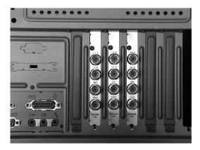
The connector on the SyncBoard that is labeled as "M" (Master), must be inserted into the Master/Slave connector of the left-most digitizer, if you are facing the BNC connectors of the ATS850 digitizers.
