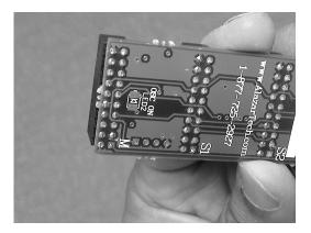
If you are installing fewer than the maximum number of digitizers supported by your SyncBoard, the unused SyncBoard connectors must be on the righthand side of the digitizers, if you are facing the BNC connectors of the ATS850 digitizers.
