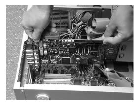
Always screw the digitizer bracket to the chassis in order to create a stable and robust connection to chassis ground.
