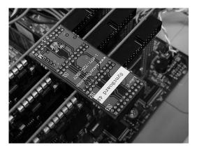
The presence of a SyncBoard is detected by the ATS850 driver when the ATSApi DLL is loaded. This DLL gets loaded when you run any application program written for ATS850. Examples of such application programs are AlazarDSO<sup>™</sup>, one of the sample programs supplied with ATS-SDK or ATS-VI or any custom software written using ATS-SDK or ATS-VI.
