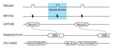
NOTE 1: Some Trigger events may be missed while data is being off-loaded from on-board memory NOTE 2: Virtually all CPU cycles are used up in managing data acquisition. Very little left for for data processing
