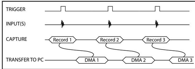
Data is returned to the user in buffers, where each buffer can contain from 1 to 8192 records (triggers). This number is called RecordsPerBuffer.
