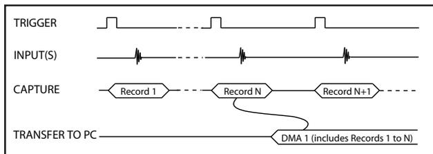
Note that a DMA is not started until RecordsPerBuffer number of records (triggers) have been acquired and written to the on-board memory.
