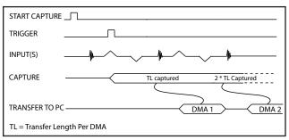
Triggered Streaming AutoDMA buffers do not include headers, so it is not possible to get trigger timestamps.
