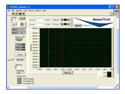
If you are programming a Master/Slave system, you can select the next board by incrementing the **Device** number (in the top-left corner) and going back to the ATS\_Set\_Device VI to setup that board. Click on **Continue** to download all the controls to the next board.
