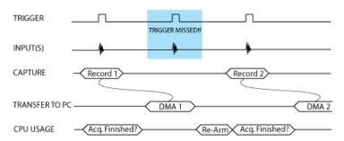
NOTE 1: Some Trigger events may be missed while data is being off-loaded from on-board memory NOTE 2: Virtually all CPU cycles are used up in managing data acquisition. Very little left for for data processing
