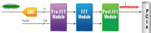
Up to 2048-point FFT length is supported. A user programmable complex windowing function can be applied to the acquired data before FFT calculation.
