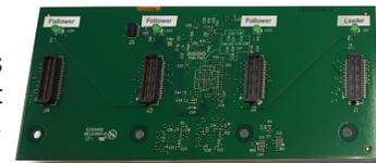
SyncBoard-9351 is available in different widths: 2x, 4x, 2x-W, 3x-W or 4x-W.
