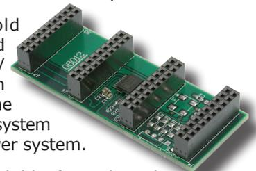
SyncBoard 310 is available for 2 board synchronization or 4 board synchronization.
