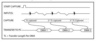
The amount of data to be captured is controlled by counting the number of buffers acquired. Acquisition is stopped by an AbortCapture command.
