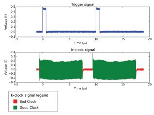
AlazarTech's *OCT Ignore Bad Clock* technology, allows safe operation with these out-of-specification clocks without requiring the use of a dummy clock in the source.
