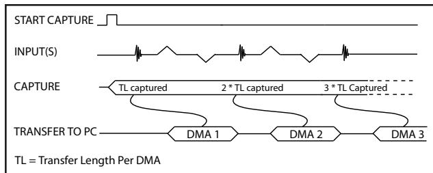
Continuous AutoDMA buffers do not include headers, so it is not possible to get trigger time-stamps.
