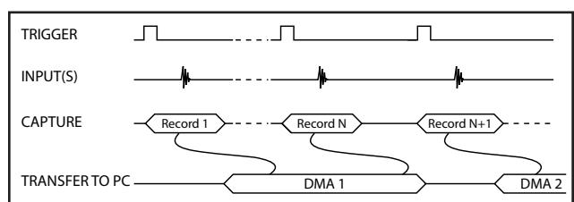
NPT AutoDMA buffers do not include headers, so it is not possible to get trigger time-stamps.
